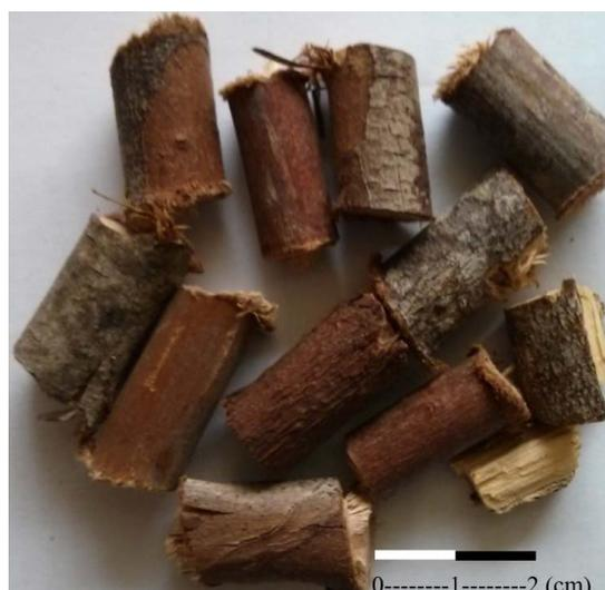
**Fig. 7** – Minced eucalyptus branch used in gasification tests. **Source:** Authors' collection.
