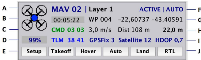
Fig. 7 – Real-time telemetry panel for each RPA.
