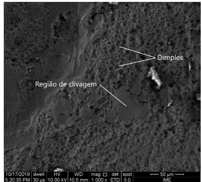
Fig. 5 – Close micrograph obtained by SEM for the fracture of steel in a tensile-tested study.
