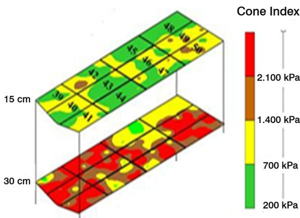
**Fig. 4** - Diagram of soil maps separated into layers with the respective mean values of CI. **Source:** [2]
