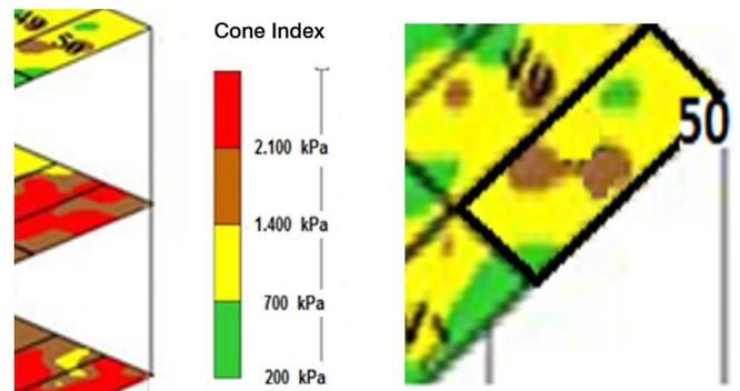
**Fig. 5** – Details of the soil map diagram separated into layers with the respective CI values. **Source:** [2]
