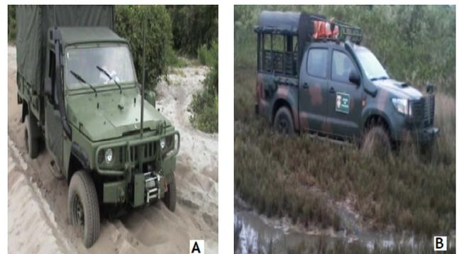
**Fig. 15** – Marruá vehicle during trafficability test in sandy soil typical of coastal region (A) and Hilux vehicle in typical mangrove soil (B). **Source:** [2]
