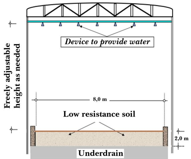
**Fig. 10** – Cross-sectional diagram of the standardized track for the trafficability test. **Source:** [2]
