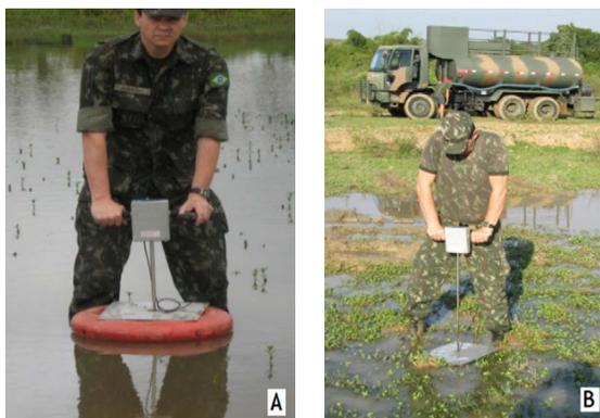
CI test with electronic cone penetrometer
