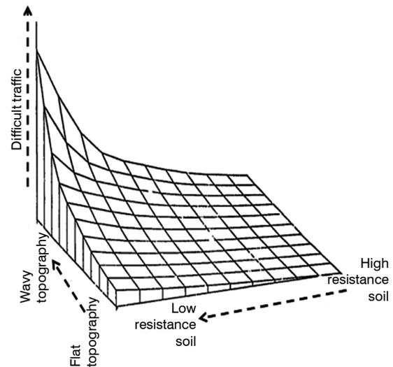
**Fig. 6** - Draft correlating soil resistance characteristics and topography with difficulty of trafficability. Source: [2]
