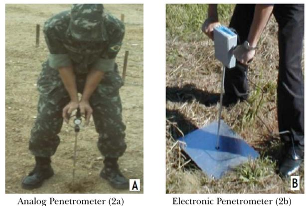
Fig. 2 - Examples of cone penetrometers. Source: [2]
