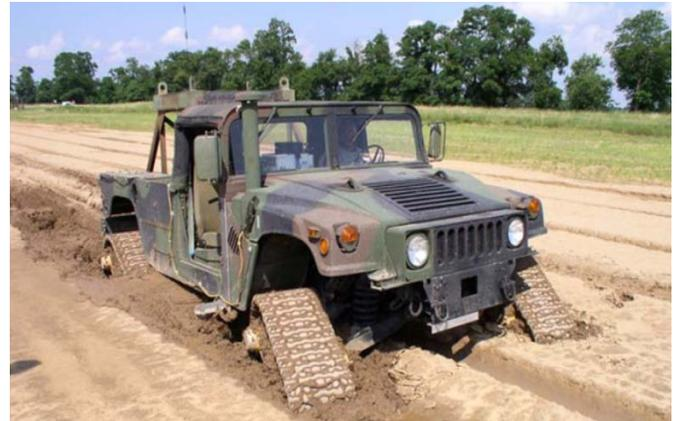
Fig. 8 – Example of traffic test being performed on artificially prepared tracks. **Source:** [13].
