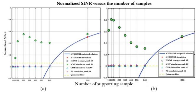
**Fig. 4 – Normalized SINR versus the number of support samples,  $K$ , of HMWF,  $M = 40$ ,  $N = 16$ , 100 Monte Carlo iterations. (a) Mobile ULA radar, rank  $r = 55$ . (b) Fixed URA radar, rank  $r = 16$ .**
