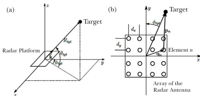
Fig. 2 - (a) Geometry of the radar platform with URA. (b) Top view.
