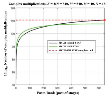
**Fig. 6 - Number of complex multiplications versus the number of stages (rank) of HMWF and MWF algorithms,  $K = MN = 640$  support samples.**
