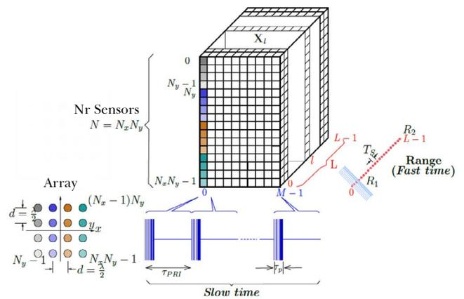
Fig. 3 - Coherent processing interval (CPI).
