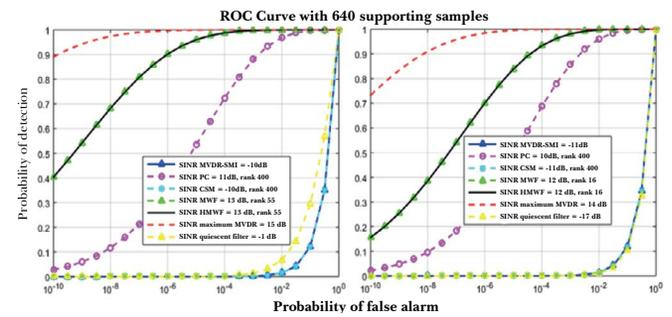
**Fig. 5 -  $P_D$  versus  $P_{FA}$  (ROC Curve),  $K = MN = 640$ , 100 Monte Carlo iterations. (a) Mobile ULA radar, rank  $r = 55$ . (b) Fixed URA radar, rank  $r = 16$ .**
