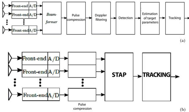
**Fig. 1 - Comparison between block diagrams of (a) a Conventional Radar Processor and (b) a Radar STAP Processor.**
