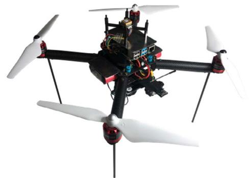
Fig. 9 – 330mm UAV built to play the role of stationary UAV.
