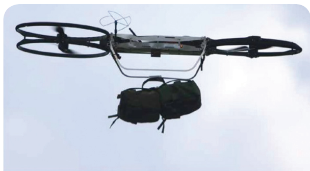
A joint tactical autonomous air resupply system carries a small package during the Maneuver Fires Integrated Experiment at Fort Sill, Okla., on April 12, 2017. This technology offers sustainers the possibility of using unmanned aerial systems to deliver supplies on the battlefield. (Photo by Monica Wood)
