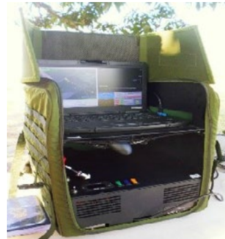
Figure 2-2 - FT-100 Ground Station
