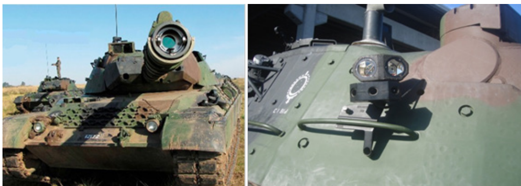
Fig 3: DSET BT/41 instalado na VBCCC Leopard 1A5
