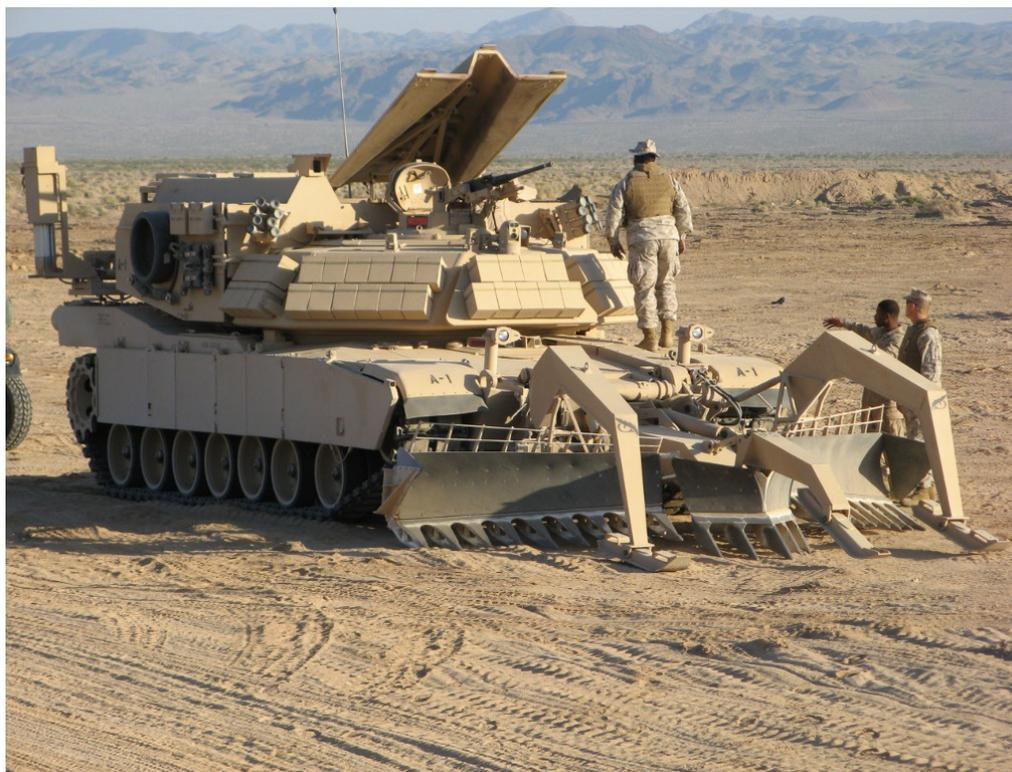
Figura 08 - Assault Breacher Vehicle (ABV)
