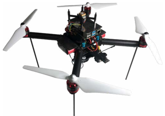
Fig. 10 – 330mm UAV built to play the role of stationary UAV.
