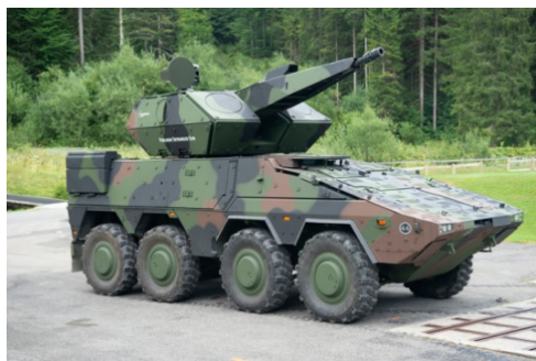
Figura 5: VBC AAe Oerlikon Skyranger (plataforma Boxer).
