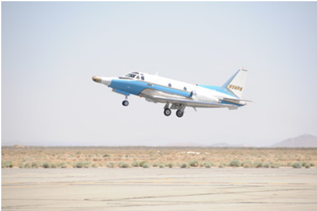
Figure 4 – Captive flight test (2015) of the multimode seeker developed by the American company Raytheon. The seeker prototype was installed on a Tomahawk nose fixed to the front of a T-39 aircraft.
