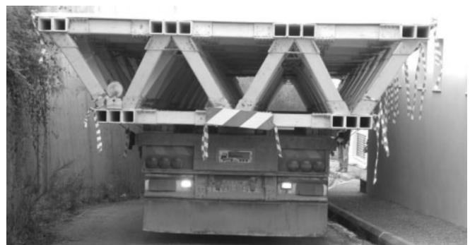
Fig. 13 – Transport of the structure on a truck. Source: [9].
