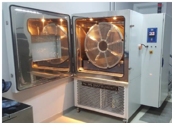
Fig. 14 - Tumbler used in the assessment of ballistic vests according to NIJ 0101.06.
