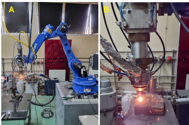
Figure 2 - Overview of deposition equipment: (A) robotic arm; and (B) laser head and powder feeders.
