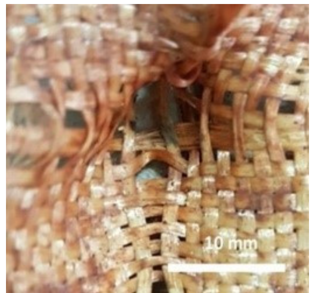
Figure 3 - Sample with 7% hematite after the energy absorption test.
