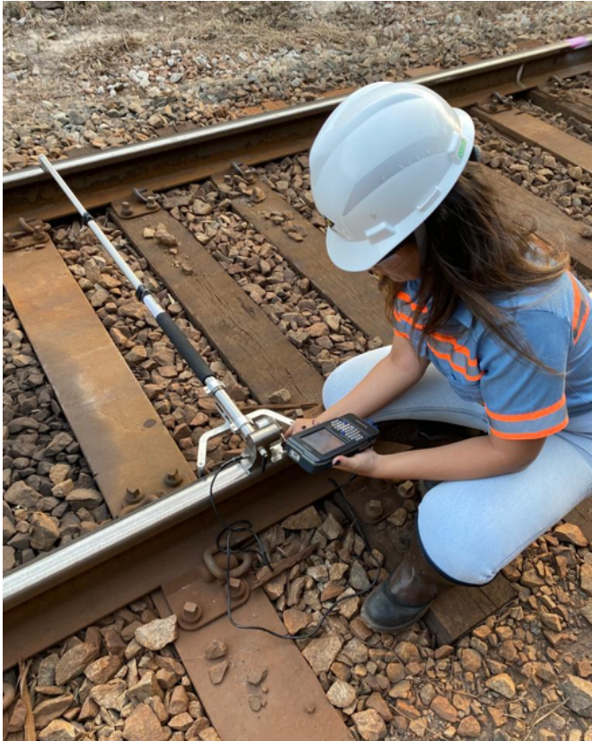
Figure 2 - Field measurement with the mini prof.
