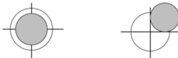
Figure 6 – The circle on the left represents a high accuracy and a low precision. The circle on the right indicates low accuracy and low precision.
