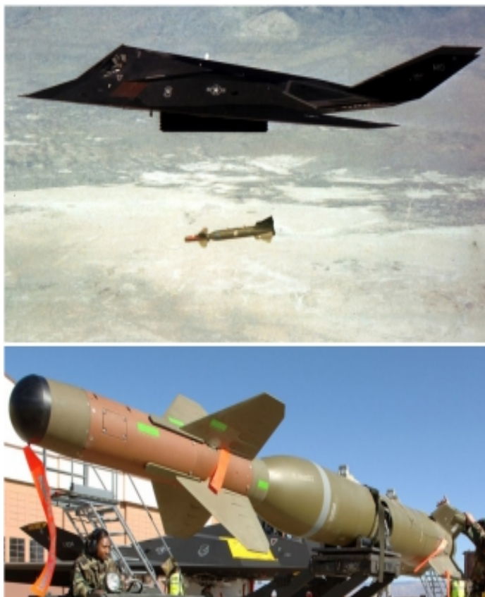
Fig. 6 - Bomba guiada GBU-27 Paveway-III com seeker laser semiativo
